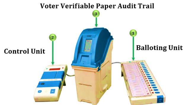
FIGURE 2 A close-up of an electronic voting machine with its Control Unit (CU), VVPAT, and Ballot Unit (BU).
